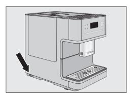
Set the main switch on the left-hand side of the machine to the "I" position. When you turn the machine on for the first time, the following message will appear in the display: "Miele - Willkommen".
